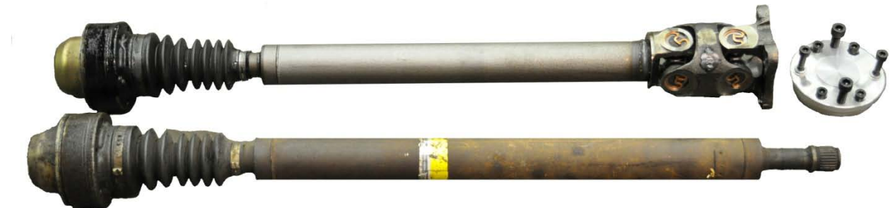
Figure 1. CCI Replacement shaft with adapter flange and mounting bolts and replaced drive shaft viewed side by side.
